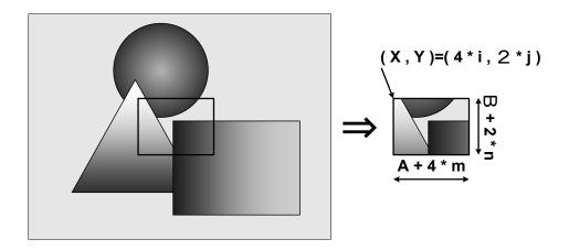
In the scalable mode, camera reads out only necessary area at the normal speed and reads out other area at high speed. The trigger interval can be shorter when the vertical height size is small.
