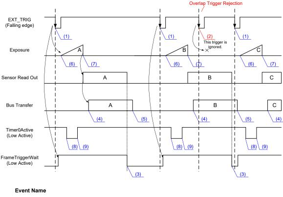
(1) FrameTrigger : Reception of Frame Start Trigger. (2) FrameTriggerError : Rejection of Frame Start Trigger. (3) FrameTriggerWait : Start of waiting for Frame Start Trigger. (4) FrameTransferStart : Start of transferring streaming data. (5) FrameTransferEnd : End of transferring streaming data. (6) ExposureStart : Start of Exposure. (7) ExposureEnd : End of Exposure. (8) Timer0Start : Start of Timer0. : End of Timer0. (9) Timer0End
