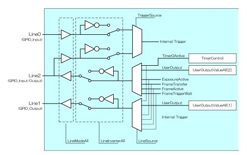
GPIO internal circuit diagram
