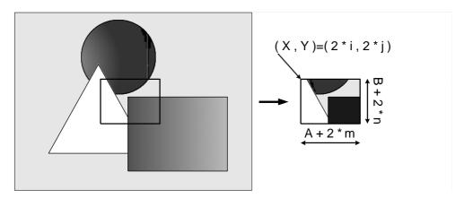
In the scalable mode, camera reads out only necessary area at the normal speed and reads out other area at high speed. The trigger interval can be shorter when the vertical height size is small. However, the trigger interval cannot be shorter when the horizontal width size is small, due to the operation me chanism of the CCD sensor.
